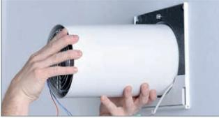
Install the inner wall panel using suitable attachment elements and carefully insert the ventilator unit (ventilator faces towards the room) into the wall. Observe that in the process the connection pipe of the ventilator is not bent / damaged. The ventilator unit can be aligned above the protection grid during the installation and be pulled back out of the wall duct again for maintenance purposes.
