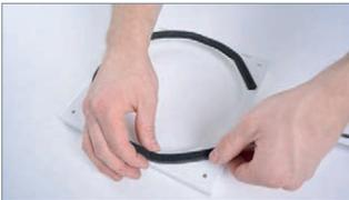
Adhere the supplied sealing tape circumferentially to the rear side of the outer wall panel.
