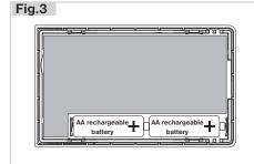
The thermostat enables backup of time in case of power failure. You must use rechargeable batteries 2x1,2 V, type AA/R6. After power failure, the time remains current (approximate service life: 2 years, according to the type of batteries used).
