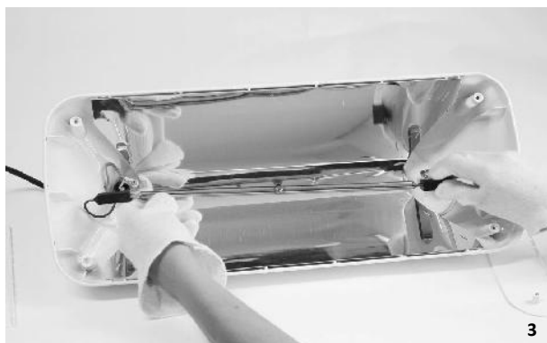
3. RELEASE THE BULB FROM THE CLAMPS.
