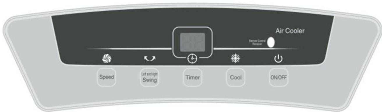
**ON/OFF:** Press once this button to make the unit ready for working. It will start up with MID in 3 seconds and then revert to work under the memorized status. If for first time use, it will start up with MID in 3 seconds and then work with LOW. Press again this button to turn OFF.
