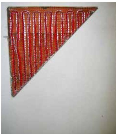
PLASTER SECTION WITH HEATER APPLIED INSIDE
