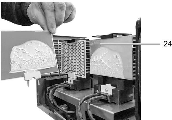
4. Apply new heat-conducting paste on the refrigeration unit (24).
