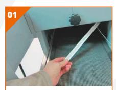
Remove the lamp, including reflector, from the process machine.
