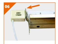
Press the top of the "spade" down until the elbow/bend sits on the same feature at the base of the reflector end clips
