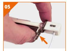
Place the retaining "spade" attached to the Victory replacement lamp over the reflector end clips.
