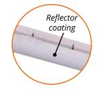
A clear, uncoated lamp emits heat in all directions. Without a reflector, a large proportion can be wasted. A reflector coating redirects heat towards the substrate resulting in improved performance and energy savings.
