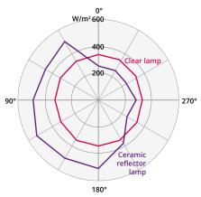
Irradiance graph shows that a clear lamp emits energy uniformly in all directions, while a reflector lamp has higher output in the 0° – 180° range (front of lamp) and reduced output in the 180° – 0° sector (rear of lamp).
