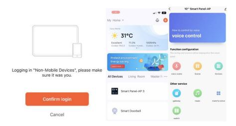
(5) Enter the panel interface in the Tuya App, you will see the gateway and switch icons like and . Click the switch icon to control 2 local switches (load of each switch for lamps should be no more than 200W.). It means the switch is off when the icon is in grey, and the switch is on when it is in orange.
