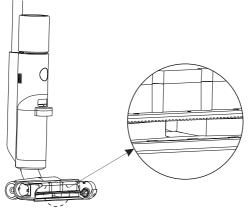
If the floor cannot be cleaned thoroughly after an extended period of use, please check whether the suction nozzle of the floor brush is blocked. When cleaning the roller brush, please remove dirt inside the suction nozzle with a clean brush or a wet cloth.
