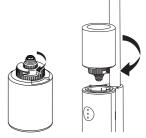
Install clean water tank on the body
