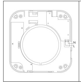
For the electrical connection of the device, L and N lines of AC 110/220V, 50/60Hz mains electricity are connected to the terminal shown in the figure on the inner wall mounting part.
