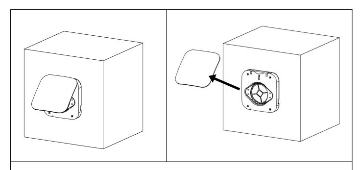
1. Remove the front cover piece by first tilting it about 45 degrees and then pulling it up from the inner cover piece.
