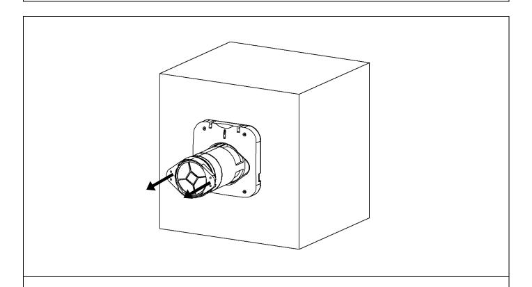
2. Remove the capsule piece by holding it from its sides and pulling it off from the pipe.
