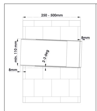
For the installation of BSK Zephyr Mini decentralized heat recovery device, a hole must be drilled on a wall facing the exterior with the dimensions indicated in the figure.
