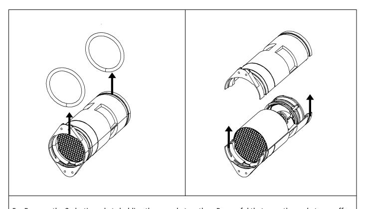
5. Remove the 2 elastic gaskets holding the capsule together. Be careful that once the gaskets are off there will be nothing holding the 2 halves of the capsule together
