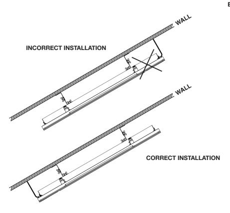
The supply cable must be at the lower end of the heater if the heater is installed at an angle or vertically.
