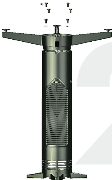
Place the table leg standing on the top bracket, so that the top bracket is facing the ground/ floor. Remove the transport protection by loosening the the two screws. Route the cord through the leg and pull it up so that it fits the table leg. Make sure the cord is positioned correctly, so that it is located directly next to the hole in the foot. Fasten the foot with the two screws.
